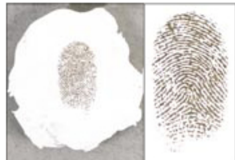
TexturLift™ lifts latent prints from soft or wet surfaces including wet paint. The lift on the left was inked before transferring the resultant print to a backing card (right).
